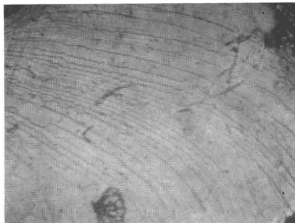
FIG. 2. Photograph of RbI crystal at a very early stage of its transformation to the high pressure phase. The near face of the crystal is in clear focus. Note the steps in the cleaved surface, the transformed "island" of surface on the back face of the crystal at the bottom of the photograph, and the island on the near surface at the upper right.
